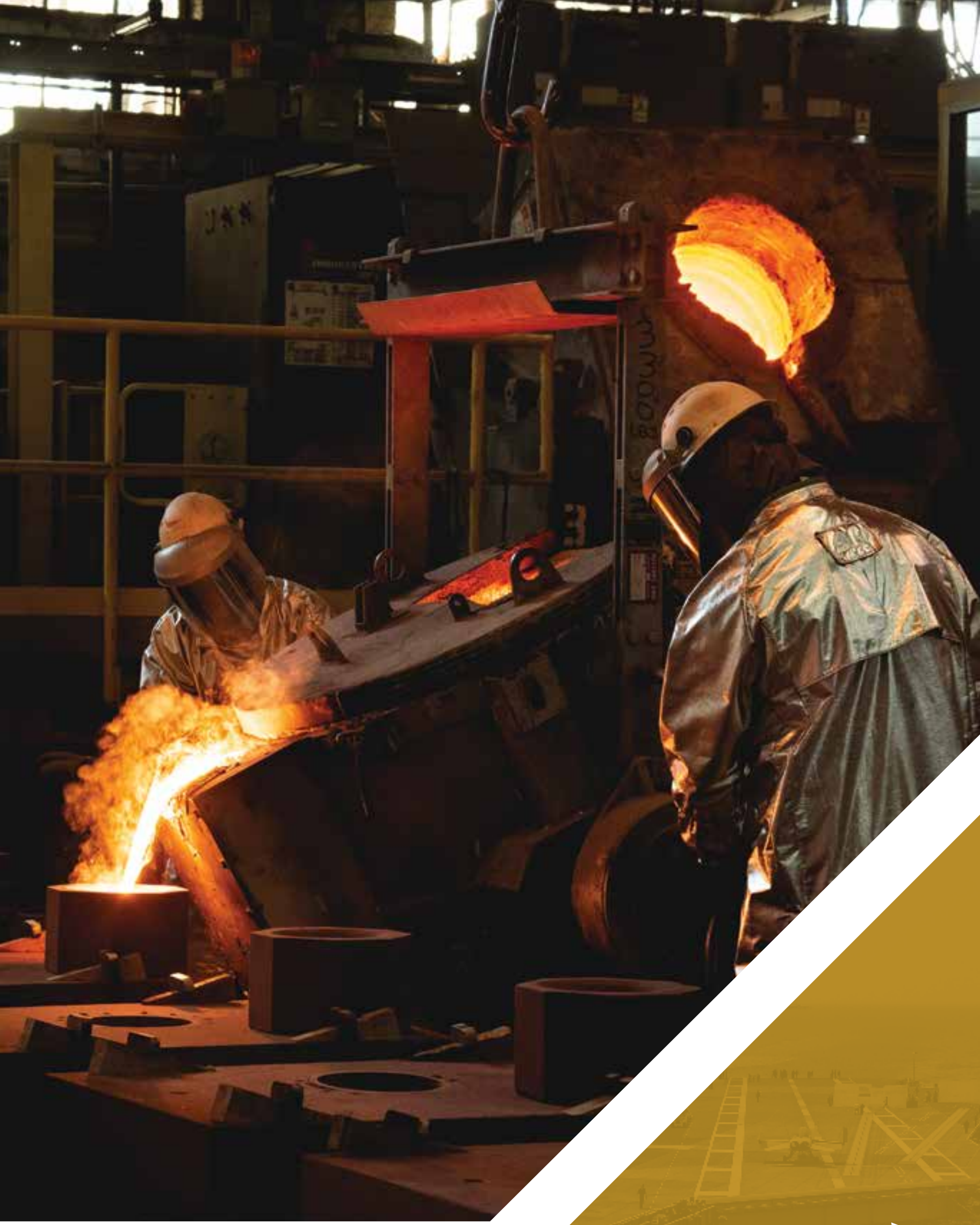
Shipbuilders pour carbon steel for a casting for Virginia -class Block V submarines Tang (SSN 805), Wahoo (SSN 806), Silversides (SSN 807) and John H. Dalton (SSN 808).
