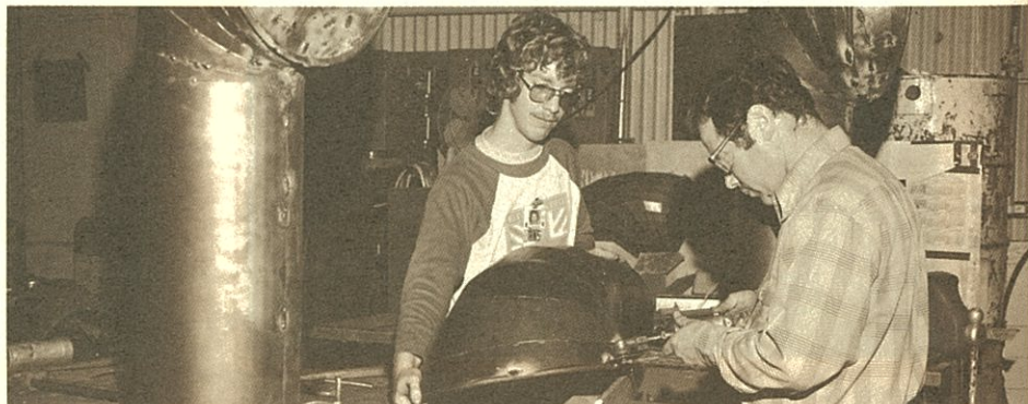
Paul Bransford, Charles Turbeville grind tack welds.
